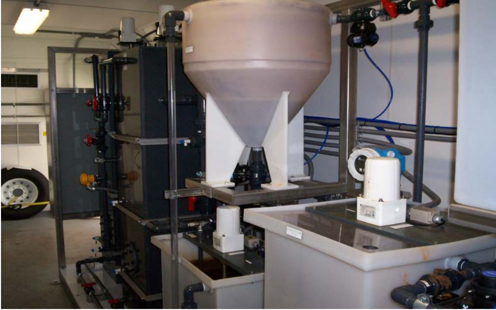
Orica Watercare magnetic ion exchange resin (MIEX) research pilot facility at South Rivanna Water Treatment Facility.
